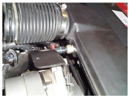
The 85100 is the mate for the MAT sensor connection. I routed the wires in the loom along the right side of the engine, and broke out of that loom with 3/8" convoluted tubing behind the alternator. The resultant 6" whip is adequate to reach around the alternator and connect to the relocated MAT sensor. (A half-inch of clearance is as good as a mile.)
