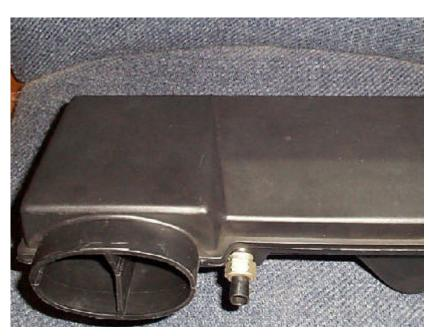
Drill a ½" hole in the resonator box near its outlet. Tap the hole to accept the 3/8" pipe thread of the MAT sensor, or install a grommet that adapts the sensor to the resonator box without leaking. It is important to maintain a seal on the resonator box, or erroneous MAF sensor readings will result in lean operation - just the thing I am tying to prevent.
