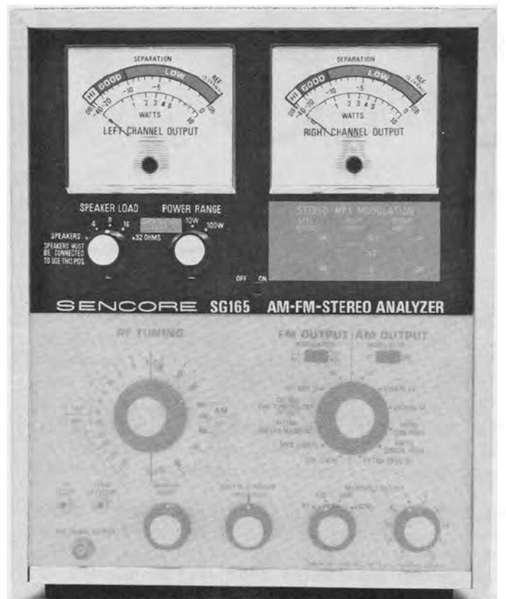
Fig. 11 Output Meters for Power Output Test
