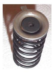
Install the screw into the spring plate and the spring over the plate. Your assembly should look like this. The flat top of the screw will bear the pressure of the spring just as the original, and the recess in the cap will prevent the screw from wandering too far from center to create problems.
