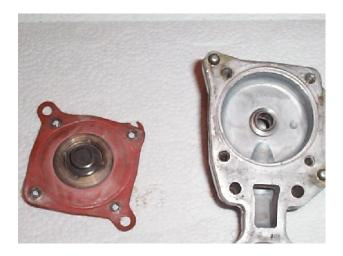
The spring/diaphragm assembly should be cleaned, then stored in a manner that will not damage the highly polished valve face on its lower side. The valve seat in the regulator body requires the same caution.
