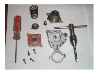
Remove the screw and spring disc from the can and unscrew the screw. At this point, you can decide whether you want to keep the original shoulder screw or replace it. You may be able to file the top of the screw flat and cut a slot to enable adjustment with a standard screwdriver. If the screw was damaged in the drilling process or you prefer a hex recess (Allen) screw for adjustment, set the screw aside.
