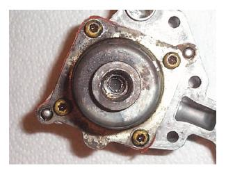
Adjust the regulator spring disc position to the same point as your original marks to begin with. Reassemble the regulator to the TBI unit in the revers order of disassembly. If there is any question about the integrity of the gaskets, replace them. Connect the fuel lines if removed and operate the fuel pump to test the system for leakage. Turning the ignition switch to the RUN position without cranking the engine should cause the fuel pump to run long enough to build pressure.
