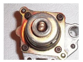
This brazed area must be drilled out to free the adjustment screw. Using the center punch, make an indentation at the center of the recess. Using this center and the inside of the recess as a bushing, drill the bronze out with a 21/64" or 'R' (0.339") drill. A 1/4" spot weld cutter also works nicely if you have access to one.
