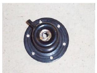
The factory powder coat finish should be cleaned from the outside of the spring cap where the jamb nut will be located. This will assure a good seal and secure attachment when brazing. It is necessary to maintain this seal since the spring cap must also hold vacuum without leaking.
