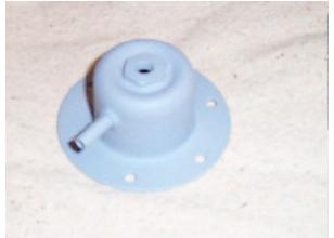
Prime the outside of the spring cap. When it has dried, sand with 400 grit paper to a smooth finish. Reprime and sand as necessary for a smooth finish.
