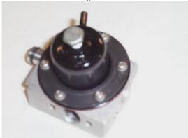
Replace the completed regulator on the vehicle. With the adjustment bolt backed out all the way, the regulator pressure should be just as it was before the conversion. To increase the fuel rail pressure, turn the adjustment screw inward. Monitor your adjustment with a fuel pressure gauge. A little adjustment should be all that's necessary, 1-2 PSIG at a time. You can verify your results with a scanner monitoring the oxygen sensor output at wide-open throttle, or your timeslips at the track.
