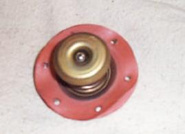
I installed a 0.310" steel ball in the recess of the regulator to receive the pressure of the screw without contacting the rod in the spring assembly. When the assembly is complete, seal the 1/4" x ½" hex bolt with Teflon tape or a liquid thread sealant, such as Permatex thread sealer. This will assure a good seal in the spring cap to retain vacuum.
