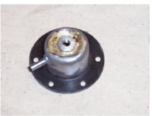
File the excess material to get a smooth finish. Clean off any flux and sand the brazed area and any burned powder coat material to a smooth finish.
