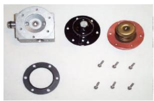
Alternately tighten the cover screws to seat the gaskets/diaphragms evenly between the spring cap and base. Tighten the screws snugly, but be careful not to over torque them. Remember that the base is die cast material.
